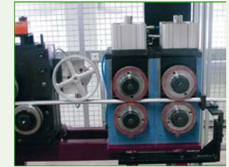
Transport unit with additional tube length encoder
