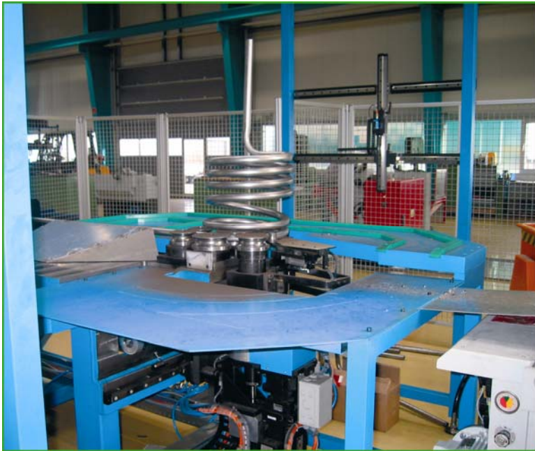
For tubes up to Ø 42 x 4.5 mm to produce tube coils, for example for heat exchangers
